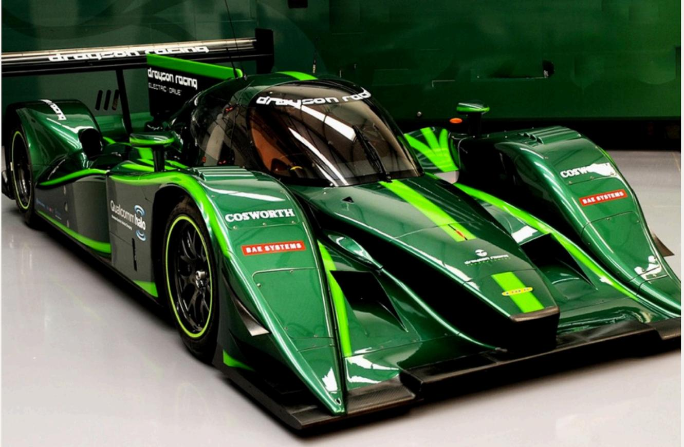
Lola-Drayson B12/69EV, zero emission 850 horsepower Le Mans Prototype car
